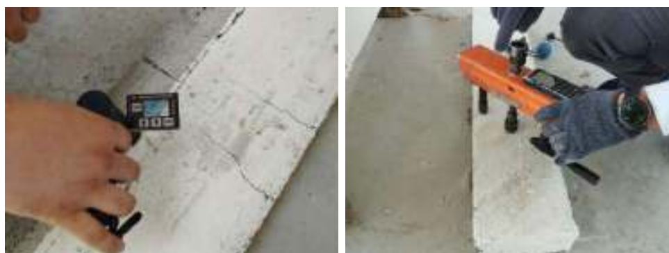
Fig. 3. Checking the practical strength of the samples
